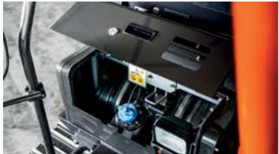
Ground access to urea tank
