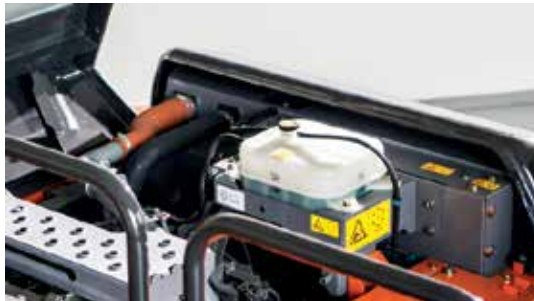
The expansion tank prevents engine parts from overheating.
